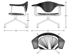
MEASUREMENT - W x D x H m Sitting height: 350 mm Seat width: 540 mm Seat deipht: 450 mm Seat height: 380 mm Chair kith: 380 mm Chair deipht: 640 mm Chair deipht: 640 mm Chair height: 700 mm Frame thickness: Ø12 mm Seat upholstered: 35 mm
