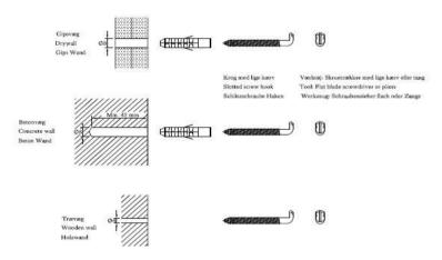
Template for drilling for mounting screws.
