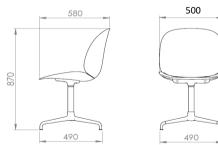
MEASUREMENT - L x W x H mm Sitting height: 445 mm Seat width: 490 mm Seat depth: 405 mm Seat height: 460 mm Back height: 430 mm Chair width: 500 mm Chair depth: 580 mm (550mm for plastic seat) Chair height: 870 mm Shell thickness: 10 mm Frame thickness: Casted Ø15-50 Front upholstered: 20 mm
