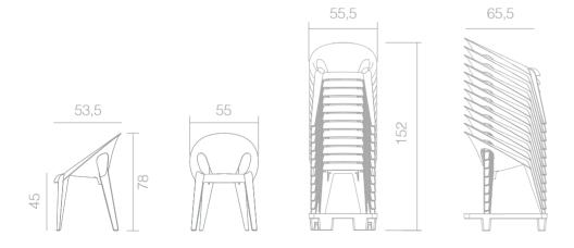
The responsibility of the design does not end with the product itself. Magis developed a logistics concept for Bell Chair to save additional resources. This entails a specially-designed reusable delivery pallet, which can stack up to 24 chairs. As a result, less packaging material is used, and the vertical stack reduces the footprint during transportation. At the same time the pallet doubles up as store display for retail partners and is made from the same recycled plastic as the chair.
