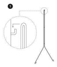
Mount the frame on the wall. Make sure the hook is fastened securely in your wall. Use an adequate wall plug or chose another hook if needed.
