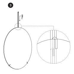
Secure the mirror. Make sure the hook catches the L-shaped screw on the back preventing the mirror from falling over.
