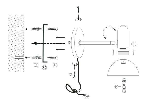
Secure the wall mounting plate (C) with screw (D) in the Plastic wall Mounts (B).
