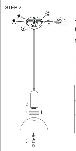
Tighten the canopy (E) with side Screw (F) to the mounting plate (C) and tighten the screw on plastic cord grip (G)
