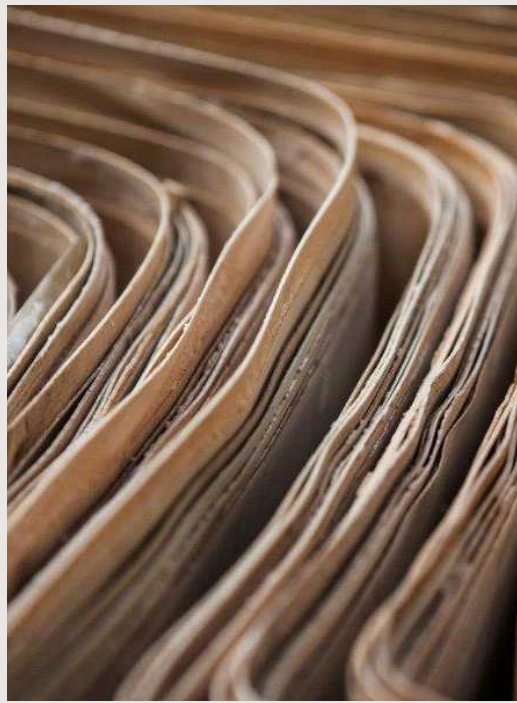
Veneer pieces 3D printed from wood waste
